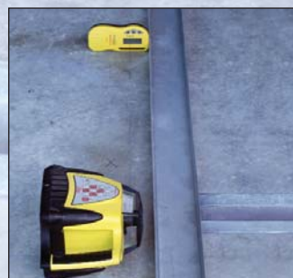
Rugby 200 with Rod-Eye Pro in a lay-down position
